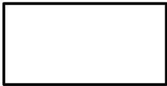
A rectangle shows a task, a step, or an activity of a process
